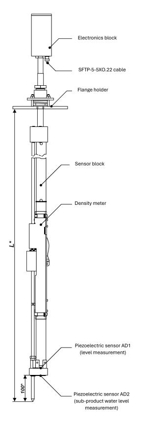
$\mathsf{L}^{\star}$  - The height of the sensor block is determined by the order (the height of the monitored tank).
