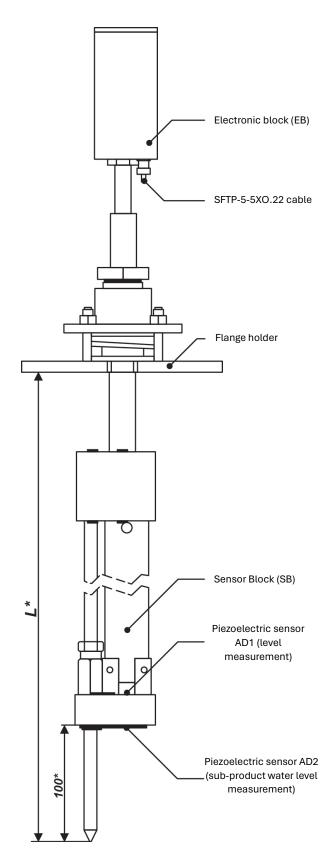
$L^{\star}$  - The height of the  $\,$  sensor block (SB) is determined by the order (the height of the controlled reservoir).
